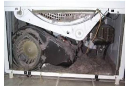
Lint accumulation in the dryer vent piping will inevitably lead to lint accumulation inside the dryer enclosure and may cause ignition from heating element
